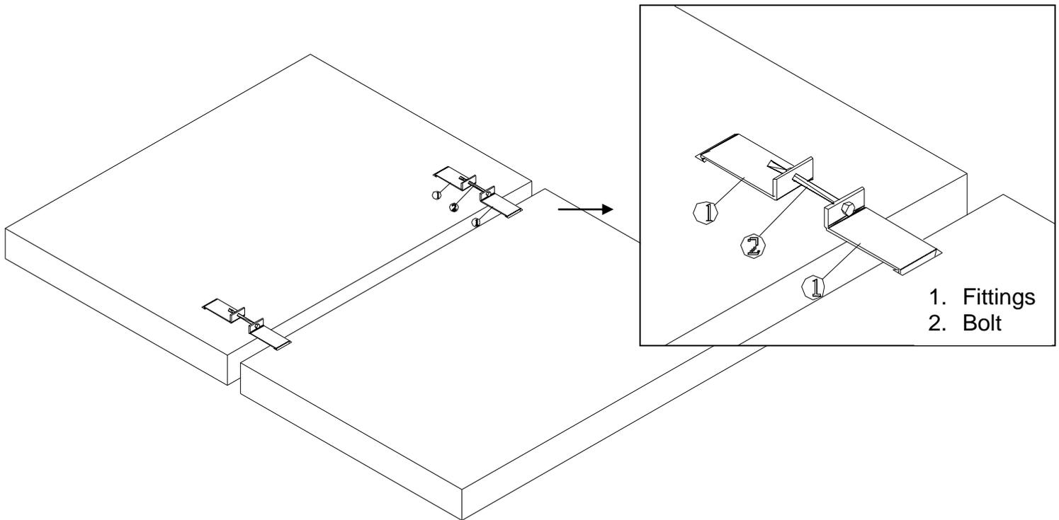
After fitting, fill rectangular track with silicone.
