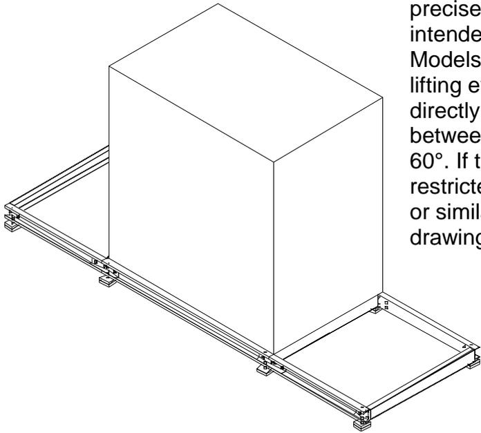
Position the middle section precisely at the centre of the space intended for the foundation. Models larger than VPM 600 have lifting eyes. If using chains or belts directly in the fittings, the angle between them must not exceed 60°. If this is not possible in a restricted space, use a lifting beam or similar equipment. See drawings (right):
