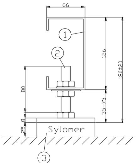
Fit the sylomer vibration dampers under the adjusting screws.
