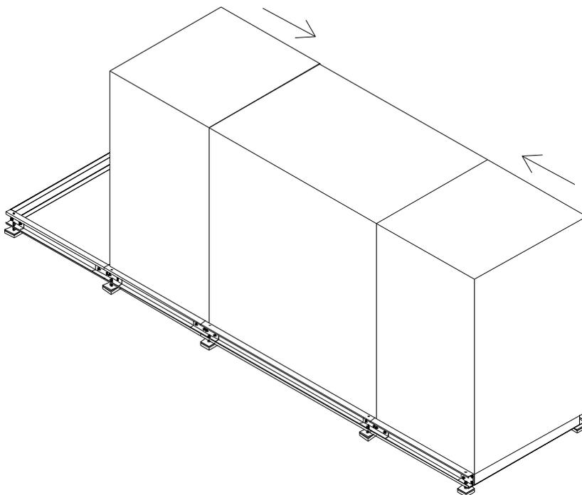
Pull the filter/fan sections into place using the enclosed fittings/bolts, with the middle section. Mount the fittings in the rectangular track at the bottom of the sections. Tighten bolts and pull the sections together. See next page.
