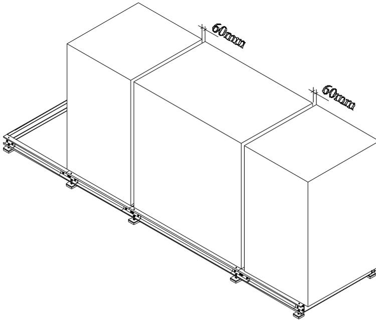
Position the filter/fan sections about 60 mm from the middle section.
