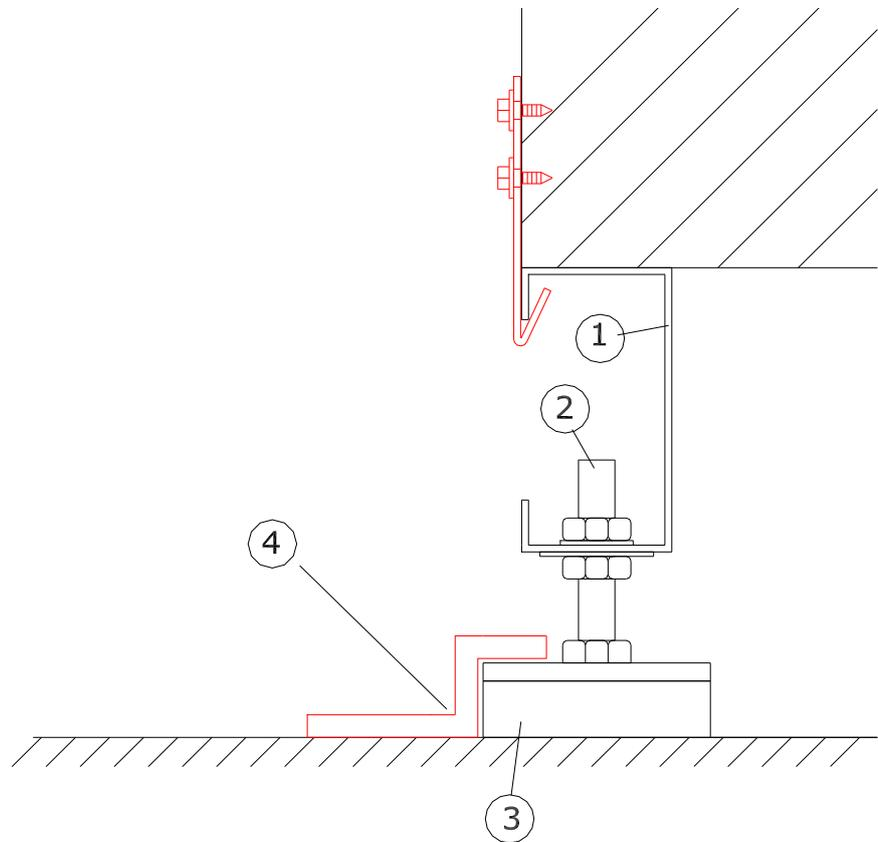
Please note that there must be space between the fitting and the feet/sylomer vibration dampers. If this is NOT the case the sylomer vibration dampers' dampening function will be impaired.
